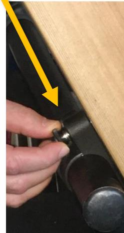
Hand tightening is sufficient !
